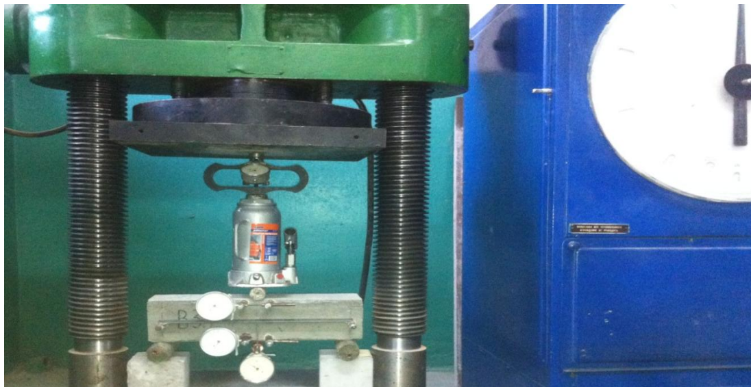
Fig. 4. Prism test according to the three-point bending scheme
