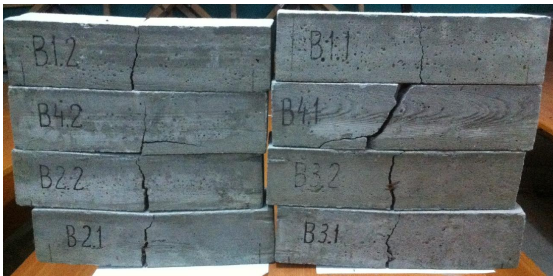
Fig. 5. Bending elements-prisms, reinforced with fibers and ribbons after tests
