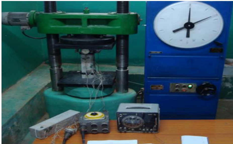
Fig. 3. Concrete prism P 1.1 during compression test
