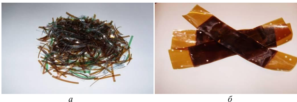
Fig. 1. Fiber (a) and strip (b) fittings made of used PET bottles
