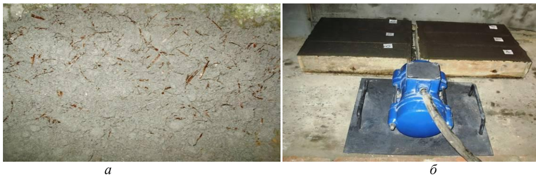
Fig. 2. Fiber-concrete mixture (a) and concrete prisms and prisms, reinforced with a ribbon of PET bottles, after manufacturing (b)
