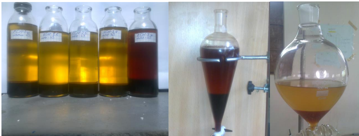
Fig. 3. Transesterification process result
