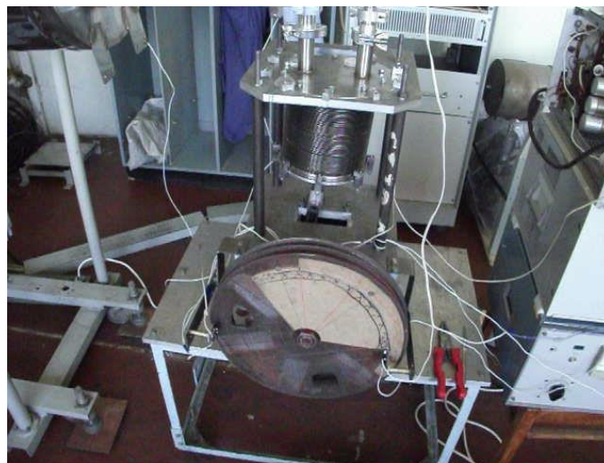
Fig. 3. Variant of the experimental sample with one working bellows
