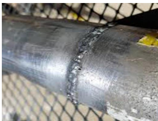
A. Crack in the welded section
