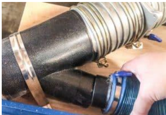
B. The iron and rubber hose connection has come loose
