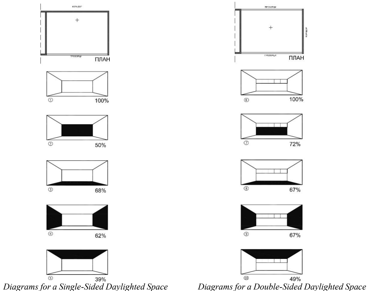
Fig. 4. Diagrams illustrating the influence of wall and ceiling colors on the natural illumination of the interior space
