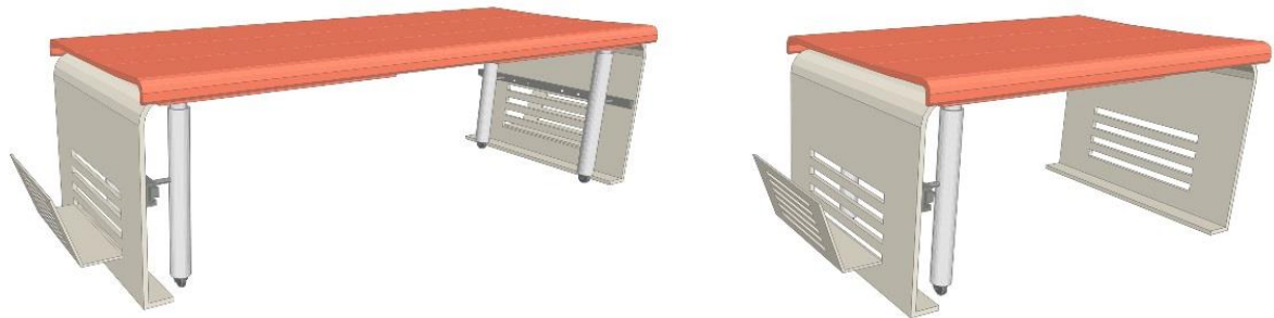
Fig. 13. Author's design of seating modules with integrated work/writing surfaces for outdoor classrooms, featuring plastic seat and tabletop
