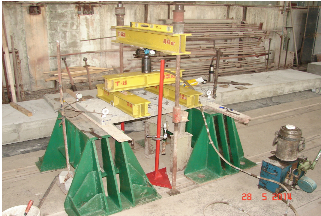
Fig. 6. General view of the slab testing stand permanent formwork.
