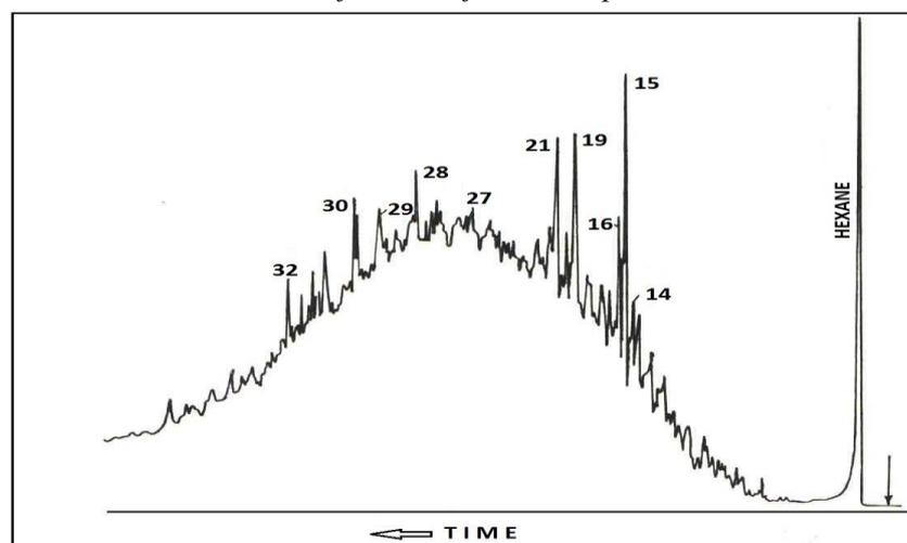
Fig. 2. Chromatogram of the 10<sup>th</sup> fraction of the TDF separation of PCP obtained from the 250-350°C fraction of Taribani petroleum. Capillary column – 60 m x 25 mm, Apiezon L, linear programming of the temperature from 100°C with a speed of 2°C/min
