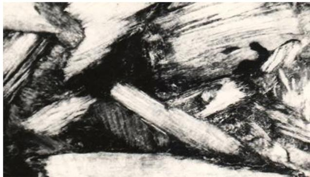
*Fig.6. The section microphoto of the arbolit sample with every filler type colored in the cross section*
