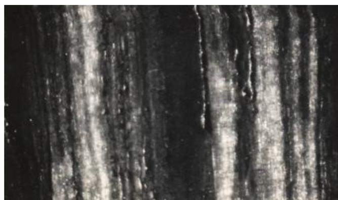
*Fig.7. The surface of the arbolit sample «fracture» with particles oriented in the longitudinal direction (magnified by 1000times)*
