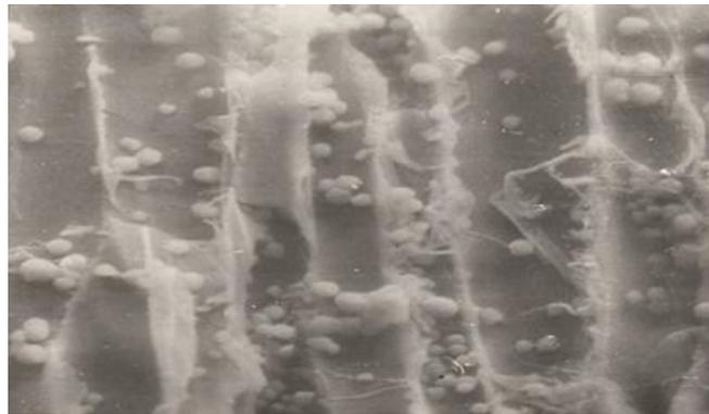
*Fig.9. The surface of the arbolit sample «section» with small particles – balls (magnified by 1000 times)*
