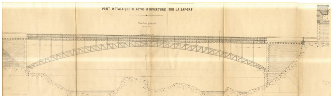
Fig. 13. General elevation of the 68.00 m wide metal arch bridge over the Safsaf river. (Archive Railway of Transport)
