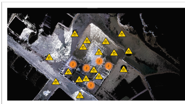
Fig. 7: Plan view of house 10 surveyed with Jet Stream Viewer (location of survey stations and diagnosis). Source : Authors.2024.
