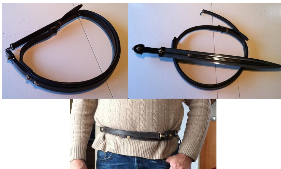
Fig.13. Georgian dagger. Damask steel. If necessary, the dagger Had the opportunity to replace the belt on the body, and when it was taken out of the scabbard, it instantly straightened out like a spring and took on its natural shape. The technology was restored by a modern Georgian master – Gocha Lagidze.
