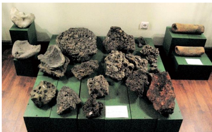
Fig.12. Metalworking waste found in smelting furnaces, which remain after smelting ore and ceramic tubes for blowing oxygen into the furnace and maintaining a high temperature. Batumi Museum.
